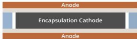
Schematic structure of encapsulated cathode
